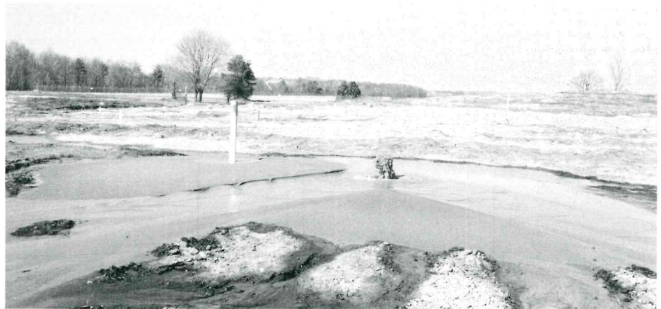
Sand boils erupting 10 seconds following blasting at the Marine Corps Training Center at the Westover Air Force Base in Chicopee, Massachusetts.
